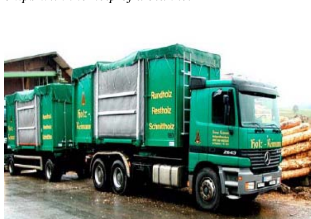
Figure 15 - Euroflat-Kombi transporting forest chips with the help of a blanket
